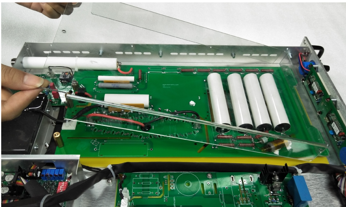
2.4.9 REINSTALL SAFETY SHIELD
