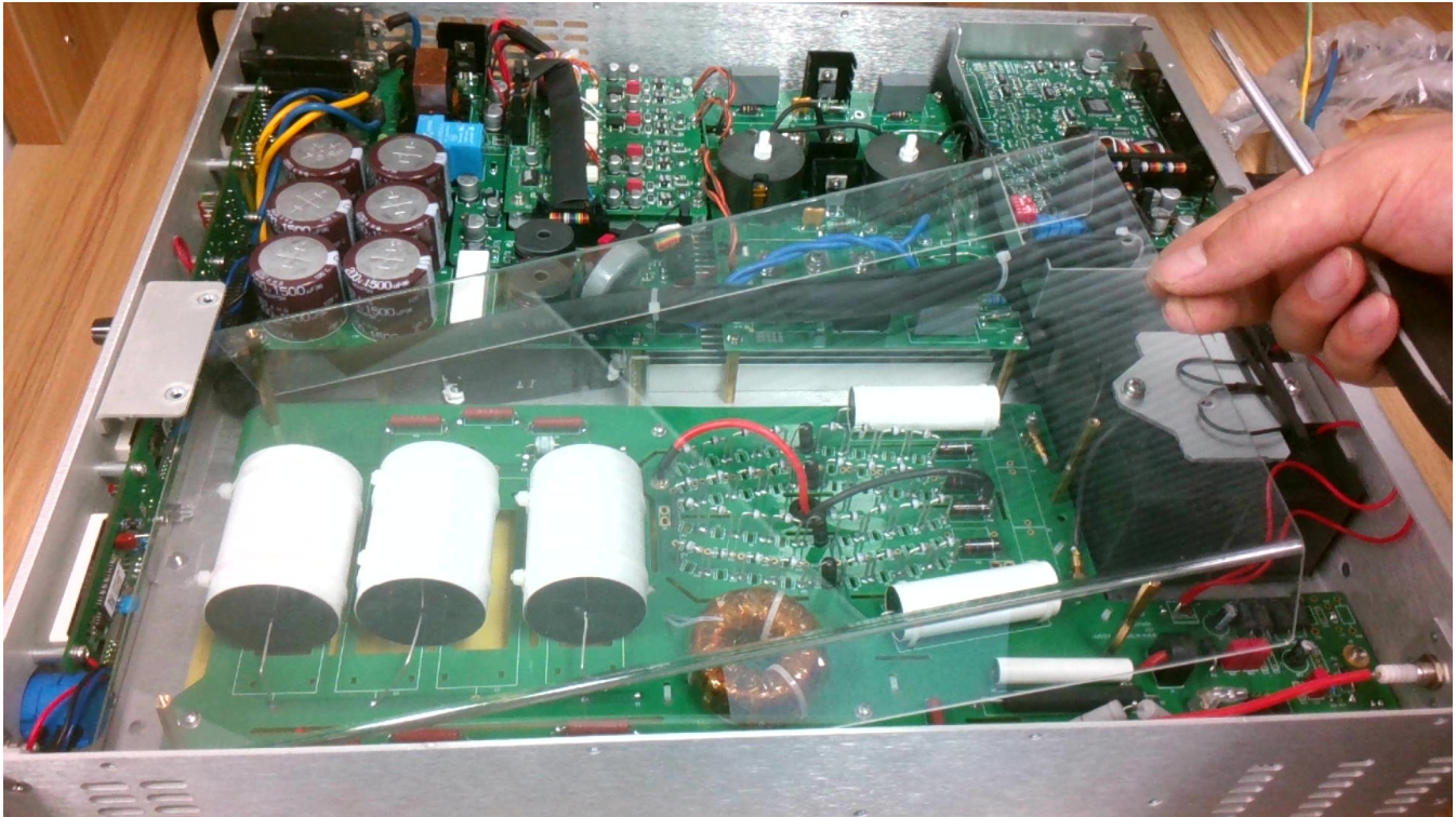
2.5.11 REINSTALL SAFETY SHIELD
